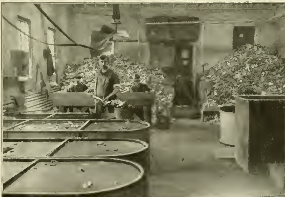
FIG. 39. Scene in a pearl button factory at Muscatine where they are soaking the clam shells in fresh water to make them less brittle.
